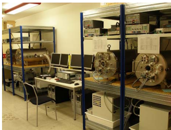
Fig. 5: PHM QM Lifetime test bench
